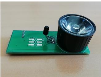
(a) The LED and the phototransistor.
