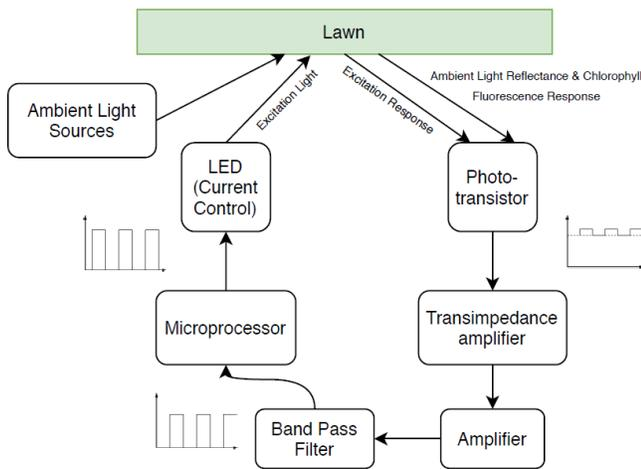
Fig. 2: The processing steps for the proposed low-cost sensor. The Microprocessor controls the LED which emits a pulsed light for stimulating the chlorophyll process. The light radiated back is then absorbed by the PT and the result further processed and sent back to the microprocessor for evaluation.
