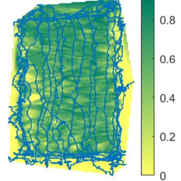
(c) The measurements positions recorded by the real-time locating system.
