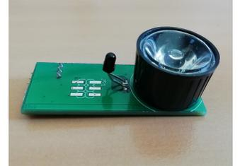
(b) The novel chlorophyll fluorescence based sensor. The main components are the LED for the illumination and the phototransistor for detecting the chlorophyll fluorescence response
