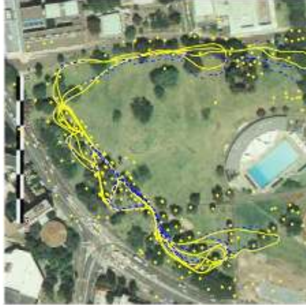
Figure 2.2: Outdoor FastSLAM evaluation from Montemerlo et al. [36] (2003): The yellow path is the estimated path of the mobile robot. The blue dashed line represents the GPS ground truth data. Features or landmarks extracted from visual data are illustrated by yellow circles.
