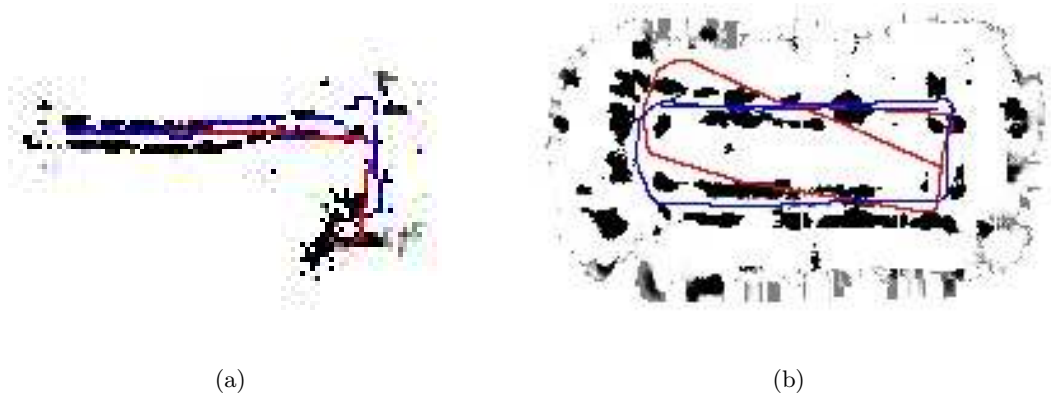
Figure 6.14: Sonar Evaluation on ICG indoor dataset: (a) Sonar Grid SLAM result after a few iterations. (b) Final map, created with sonar grid SLAM, using 100 particles. The red trajectory denotes the odometry path and the estimated robot poses are indicated by blue points.
