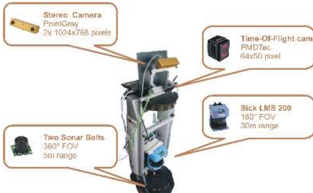
Figure 6.12: [Mobile robot used for the experiments at ICG: This mobile robot is equipped with two sonar belts, a Sick LMS 200 laser range finder and time-of-flight camera from PMDTec. The stereo camera was not used for this work. FOV means field of view.
