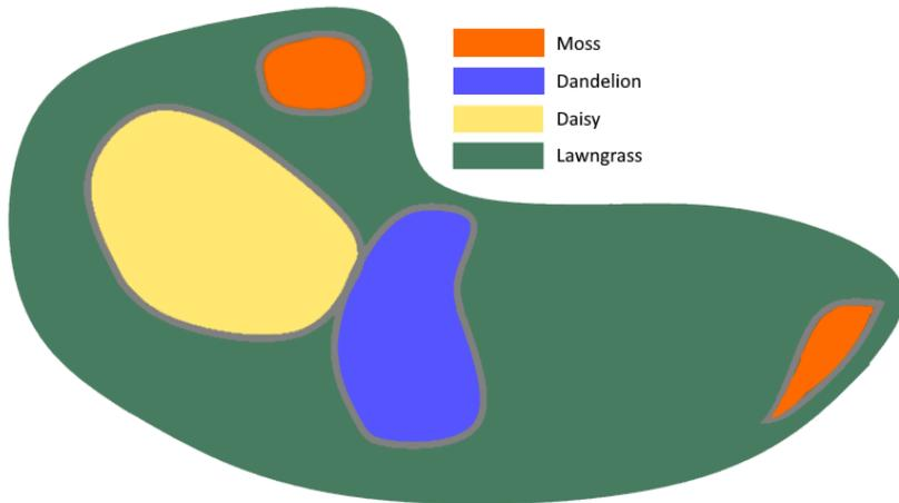
Figure 1.1: Diagram showing a possible map created by the lawn mower robot using a plant classification sensor.
